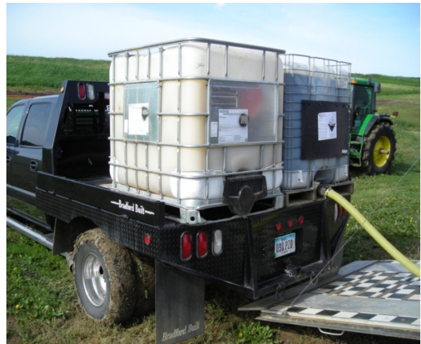
Kemira tote w/4512 Polymer & Ferric Sulfate
