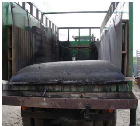
Bag supported on trailer with pallets underneath and on side. Drainage “gutter” pipe on right side.
