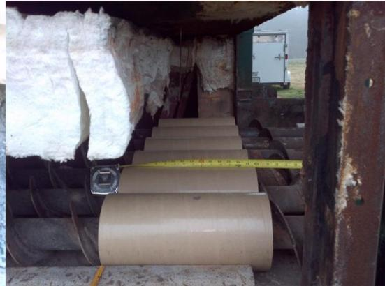
Augers are sleeved to reduce clearance and rogue air from entering gasifier
