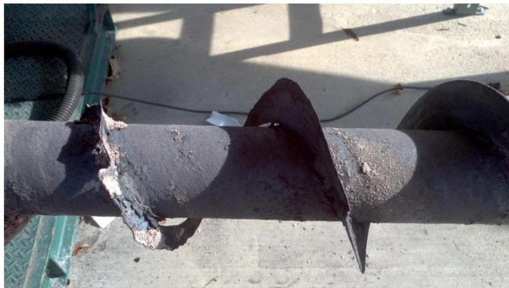
Auger flight damage evident on ash end
