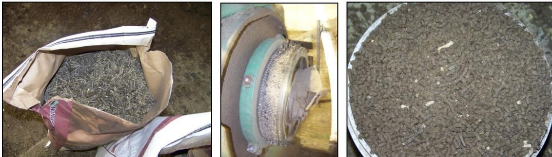
The one inch thick die made a significant improvement in the operation of the pellet mill. A wider range of biofibers moisture could be processed, and the pellet mill ran successfully on a sustained basis. From the trials, it is estimated that approximately 500 lbs of pellets could be made an hour, or 12 ton/day if operated continuously.
