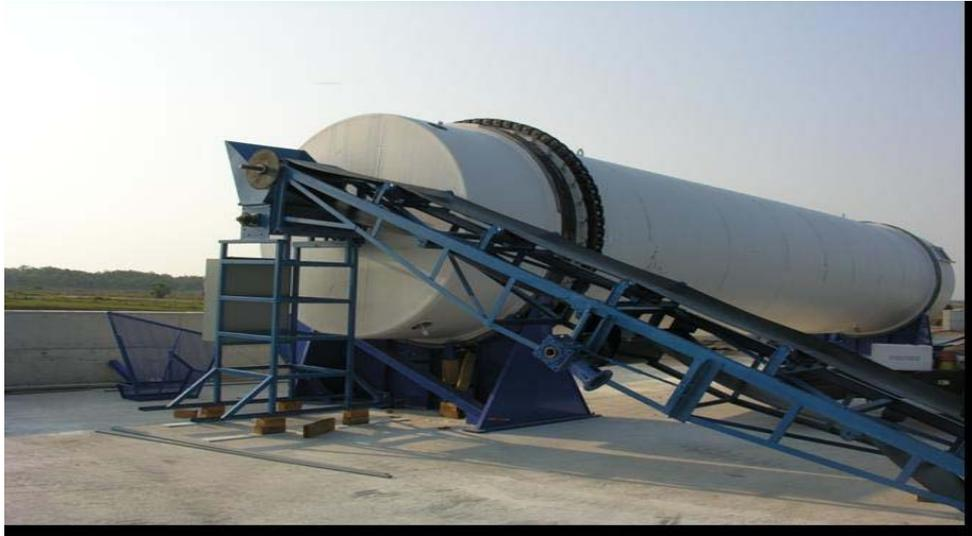
Photograph - shows the in-vessel composter utilized for processing dairy manure
