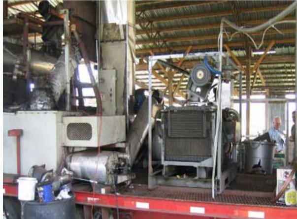
Figure 1. To the upper left is the new char screen assembly with the new heat exchanger beneath it. To the right is the char burner and associated hot air ducting installed in place of engine/generator set.
