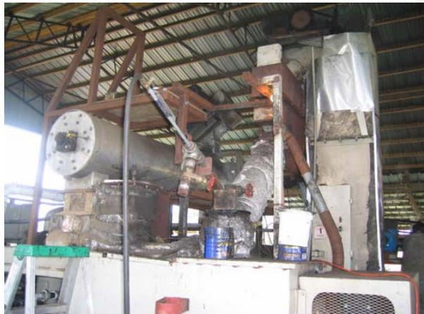
Figure 4. Old char screen assembly with old heat exchanger
