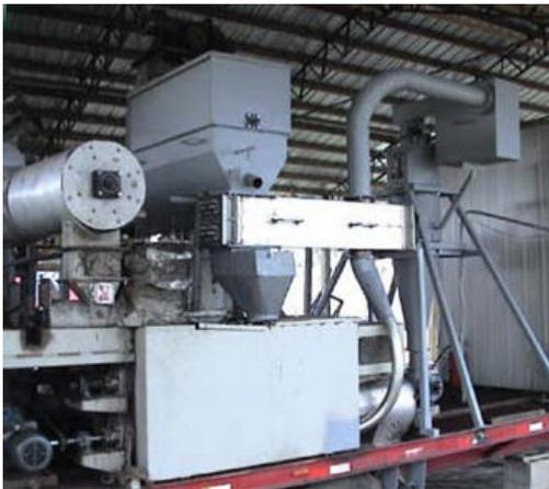
Figure 3. New char screen assembly with new heat
