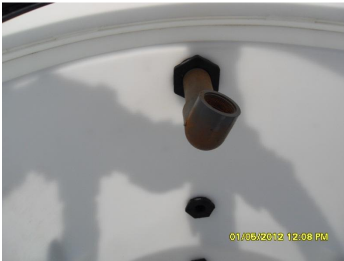
Feed nozzle in separator
